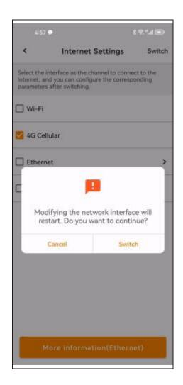
Different versions of the gateway have different options for connecting to the Internet. Users can select 4G and click "Switch" to change the connection options.
