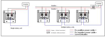
1a. For CPS SCE3.6/4.6/5/6KTL-60/120-EU inverter: If inverter connects to single battery unit or the first one of multiple networking battery units, connect the COM cable for SCE inverter to COM port of inverter and PCS port of battery unit according to cable marks, for the remaing networking battery units, choose standard Ethernet cable with the same connectors,
