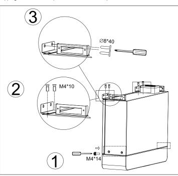
4. Fasten power control module onto the battery extension module. Then insert dust plugs into all the screw holes on the both sides.
