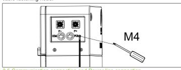
3.5 Communication connection and Power line connection
