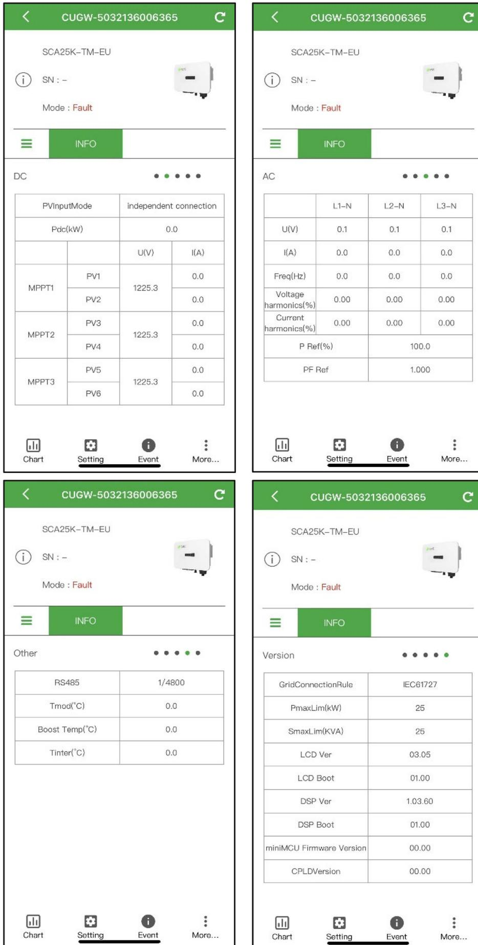
The figure displays four screenshots of the main menu for the SCA25K-TM-EU device, showing various information sections. Each screenshot includes a header with the device ID 'CUGW-5032136006365', a refresh icon, and a status bar with 'Mode : Fault'. The 'INFO' tab is selected in all views.
