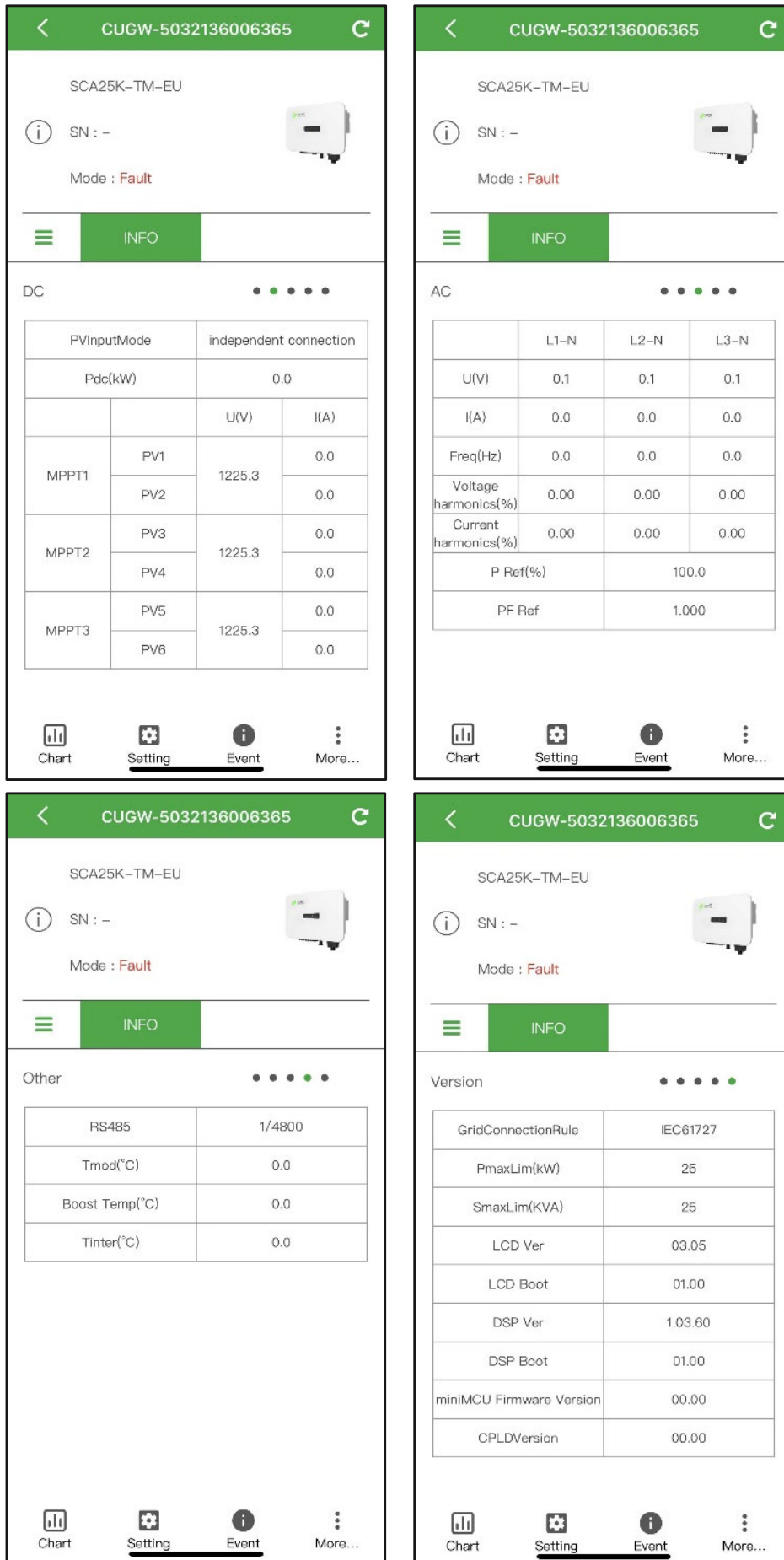
Figure 6-2 Main information on Main Interface
