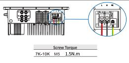
Lock the AC cable to the corresponding AC terminals.
