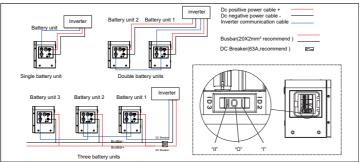
1. Insert communication cable to BMS port of inverter and PCS ports of battery
