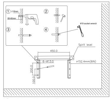
2. Fasten the base module onto the wall bracket. Tools: M8X16 combination screw and M6 torque screwdriver.
