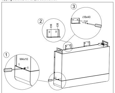
4. Fasten power control module onto the battery extension module. Then insert dust caps into all the side screw holes, repeat this operation on the oppsite side till all the side scew holes are plugged up.
