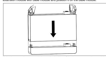
3. Lock screws into screw holes on both sides of the battery extension module, to ensure extension module is securely installed on the base module; fasten wall anchor on the battery extension module, and then fasten it on the wall. Similarly, install other battery extension modules in turn and fasten them.
