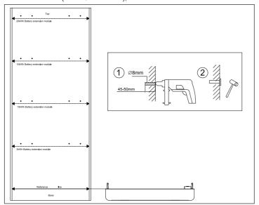
2. Two people jointly lift the battery extension module, align the battery extension module with base module and position it on the base module.
